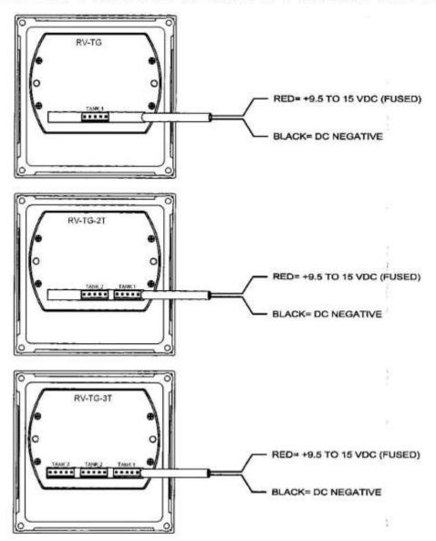
The LED Tank level gauges provide an economical and simple tank monitor of 1, 2 or 3 tanks. The tank gauges can only be used on fresh and grey water and are not suitable for black water or fuel
